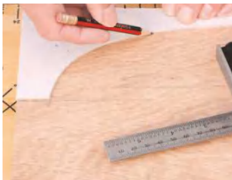
STEP 17. Draw around the template on both brackets, and then cut these carefully with a bandsaw or jigsaw
